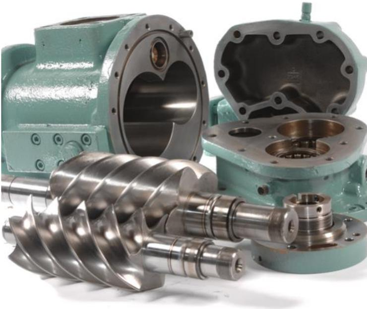
After disassembly, we dip our compressor bodies in acid to remove all old debris and paint, this brings the body back to as new condition.
