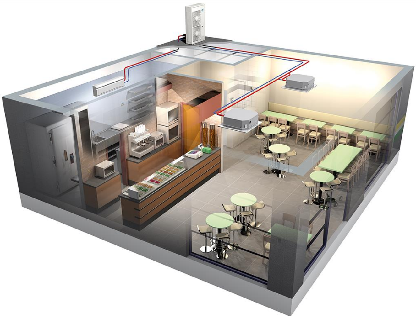
Example of a VRF system installed in a small deli / restaurant.
